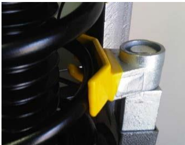
Correct hook engagement on spring coil.
